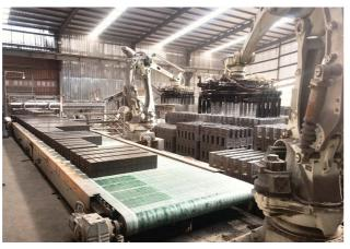
Recovered sludge used for brick production at the BOE Ordos Gen 5.5 TFT-LCD production line
